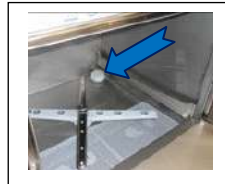
Check and refill the salt reservoir, with granulated salt (►10) ( only on machine with integral softener )
